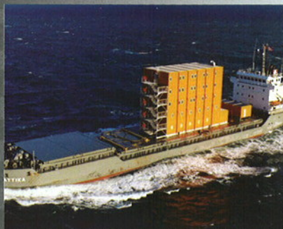
LB 4000 LQ & CHANGE ROOM MODULE DURING TRANSPORTATION
